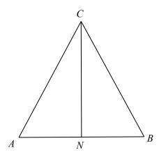
Since AC=BC, then CN is perpendicular to AB. Since BC=5 m and  $NB=\frac{3\sqrt{2}}{2}$  m, then by the Pythagorean Theorem,
