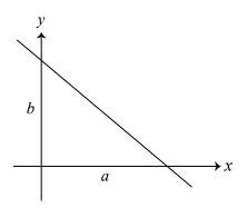
Then the area of the triangle formed by the line and the axes is  $\frac{ab}{2}$ .
