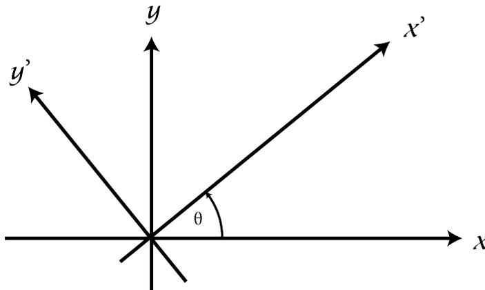
We assume that the new axes are also orthogonal. If we know the angle of rotation then we can relate the two sets of co-ordinates.
